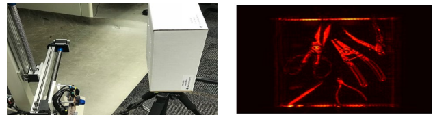
Figure 2. Left: Imaging scenario with multiple objects concealed in a cardboard box. Right: Reconstructed image.
